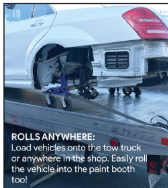
BECOMES PART OF THE VEHICLE: No need to employ any unstable or dangerous lift points. Mounts to the sub frame or cradle using the original mount points and hardware.
